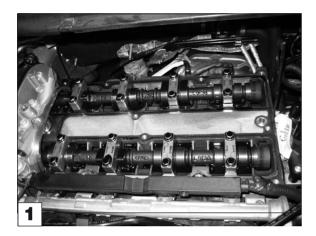
The Ford 1.6 16v. Ti VCT Duratec (Sigma) petrol engine was first introduced in the Ford Focus in 2004. The engine has variable camshaft timing (VCT) on both the inlet and exhaust camshafts.
