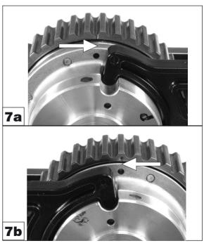
Fit AST4931 VCT Setting Plate on to the VCT Units and check that the timing marks on the **VCT Units and camshaft sprockets** align and are near to the outer edges of the Setting Plate upper arms.
