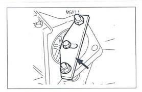
AST4834 Flywheel Locking Tool Set includes a Main Plate and 3  $\boldsymbol{x}$  inter-changeable Adaptors.
