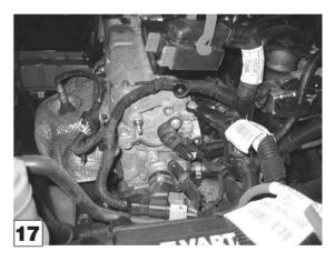
It is essential that the camshaft sensor entry hole is positioned correctly relative to the camshaft. Therefore alignment of the camshaft cover must be accurately achieved using AST4954 Fixture.
