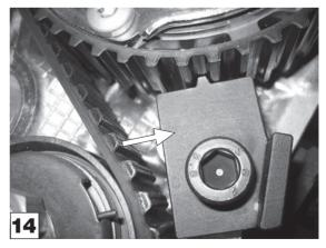
Fit AST4953 Camshaft Sprocket Locking Tool to the engine, fitting the Tool into the teeth of the camshaft sprocket, and secure with the bolt supplied in the Kit. Tighten the bolt firmly.
