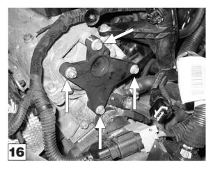
To achieve correct alignment of the cover and cylinder head, the AST4954 Fixture is secured in place at 4 locations (2 on the cylinder head and 2 on the camshaft cover).
