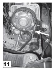
Undo the camshaft sprocket bolt cover and remove it. **NOTE:** Be prepared for oil to leak out.
