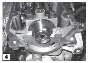
**NOTE**: The Setting Plate locates in to a "timing slot" in the rear of the camshaft.
