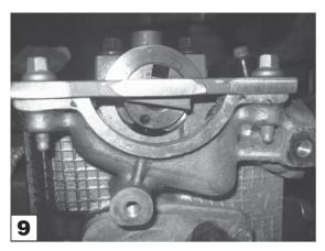
Rotate the crankshaft to engine timing position and check the camshaft timing is correct by temporarily inserting AST4952 Setting Plate in to the "slot" at the rear of the camshaft, ensuring the camshaft position is not 180 degrees out.
