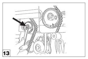
Tension the timing belt by turning the tensioner **anti-clockwise**, with Adjuster AST4513 and **apply maximum tension**. Tighten the tensioner nut.
