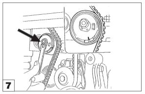
Fit AST4513 Tensioner Adjuster to the tensioner and maintain its position whilst slackening the tensioner nut. Allow the automatic tensioner to achieve a position where the front fork is aligned with the rear fork. Tighten tensioner nut to specified torque – 25Nm.
