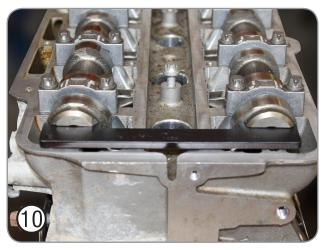
Using a spanner on the machined hexagon, adjust the position of each camshaft so that the slots in the rear of the camshafts are horizontal and above the surface of the cylinder head. Install **AST5091** camshaft setting plate.
