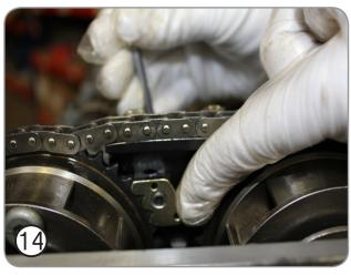
Adjust the locking wedge until it is fully located in the teeth of the inlet camshaft sprocket, then tighten the bolt to lock the wedge and sprocket in position.
