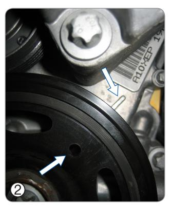
Rotate the crankshaft in the direction of engine rotation until the mark on the crankshaft pulley is aligned with mark on the engine.
