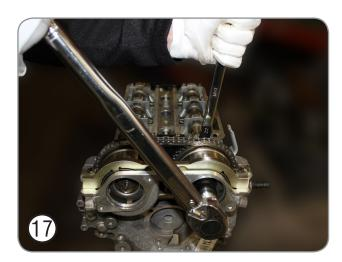
Using a spanner on the machined hexagon of the Exhaust camshaft as a counter hold, tighten the central bolt of the camshaft sprocket to **50Nm**.
