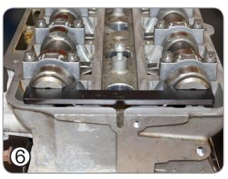
Install **AST5091 camshaft setting plate** into the slots at the rear of the camshafts.
