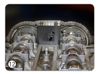
Remove the timing chain guide from the cylinder head. Install **AST5094 camshaft sprocket holding tool** to the cylinder head, leaving the 2x retaining screws and 1x locking bolt loose.
