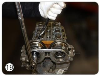
Using a spanner on the machined hexagon of the **Inlet** camshaft, counter hold and tighten the central bolt of the camshaft sprocket to its final torque value (50Nm + 60°).
