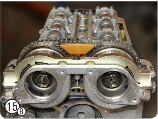
Install the appropriate VVT/camshaft sensor setting tool. Use **AST5092** for **1.0L** (3 cylinder) engines. *Picture 15A* Use **AST5093** for **1.2L** / **1.4L** (4 cylinder) engines. *Picture 15B*
