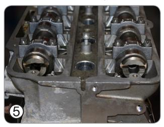
Check the position of the slots in the rear of the camshafts. With no.1 cylinder at TDC position, the slots will be horizontal and above the surface of the cylinder head.
