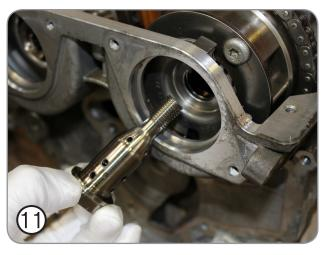
Replace the Camshaft sprocket central bolts, ensuring that the VVT units and sensor discs are free to rotate on the camshafts. Apply a small amount of clean engine oil to the flange of the new bolts before fitting to avoid rotation of the sensor disc during the final tightening procedure.
