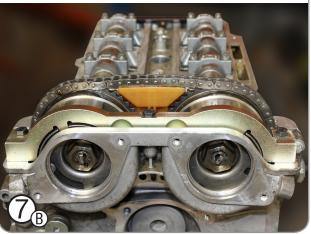
Select and install the appropriate VVT/camshaft sensor setting tool: **AST5092** for **1.0L** (3 cylinder) engines. *Picture 7A* **AST5093** for **1.2L** / **1.4L** (4 cylinder) engines. *Picture 7B*
