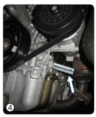
Install **AST4487 crankshaft locking pin** fully into the engine. Ensure that the crankshaft is locked at TDC position.
