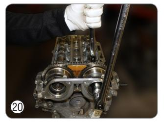
Using a spanner on the machined hexagon of the Exhaust camshaft, counter hold and tighten the central bolt of the camshaft sprocket to its final torque value (50Nm + 60°).
